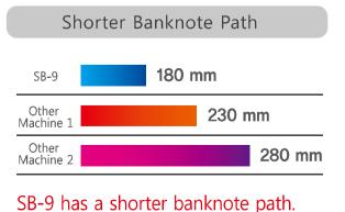
SB-9 has a shorter banknote path. The shorter the path, the less jamming.
